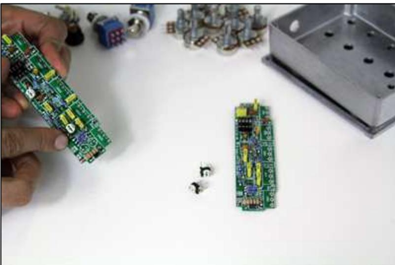
(11) Next up are the trimpots for DEPTH and PRESENCE. These three legged components should click into place. The 105 denotes 1M and the 103 is 10k.
