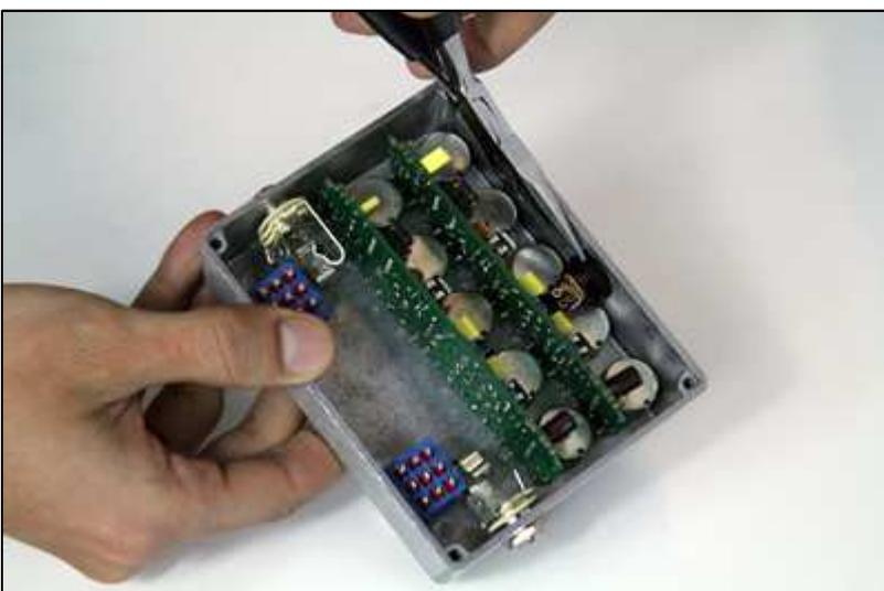
(23) Last step is to load the DC jack. Be sure to load it in as shown and tighten with the included black nut with needle nose pliers. Some inwards pressure will need to be to the outside barrel of the jack whilst fastening to ensure the jack doesn't rotate.
