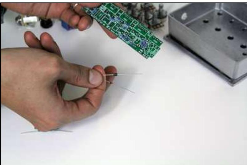
(5) There are two kinds of diodes: the orange 1N914 and black 1N4004. Diodes are polarised i.e have a positive and negative end. The negative end is marked with a black (1N914) and silver (1N4004) band. The PCB has a marking alongside the D01 for example showing which direction the band should be facing. Load in the diodes, solder and trim.
