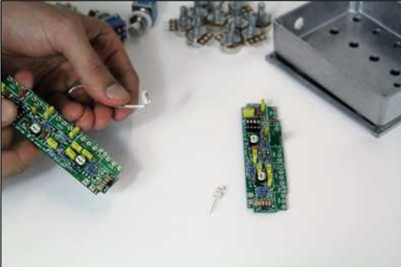
(12) Next components to load are the channel LEDs. These light-emitting diodes are polarised; again the long leg of the LED indicates the positive side.
