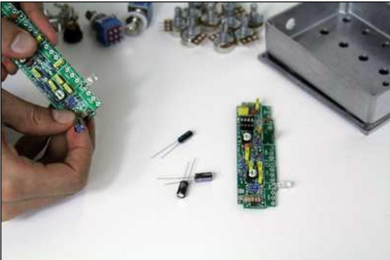
(13) The electrolytic capacitors are next to load. These are polarised, again '+' marked by the long leg, and on the opposite side is a '-' strip printed on the side of the capacitor. Take care in ensuring these are loaded in the correct orientation. Load, solder and trim.
