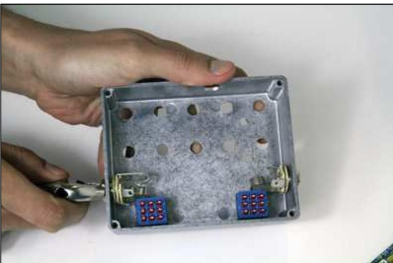
(20) Next we will load in the jacks. The input jack (shown on the left hand side being tightened) is a stereo jack with a tip, ring and sleeve orientation. The output jack is mono and has only a tip and sleeve connection. Load and secure with the included nut and washer.
