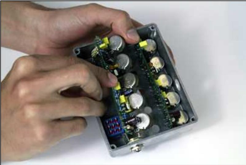
(21) Time to load in the PCBs, start with the top board (PCB A) and then the bottom board.
