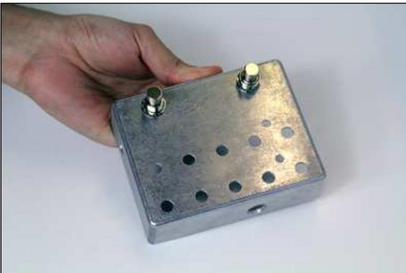
(19) Holding the footswitch in place, fasten the switch with the washers and nut on the opposite side with a wrench or socket.
