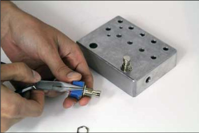
(18) Starting with the footswitch, before loading the footswitches, remove the nut and washers (plastic and tooth) and screw the final nut down to its base (shown).
