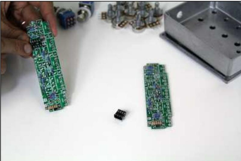
(7) Now place in the IC socket. The orientation of the socket, therefore the IC, is very important as each pin has a different function. The PCB layout has a white outline for the socket with a small notch at the top. This notch is found on the socket and indicates the direction.
