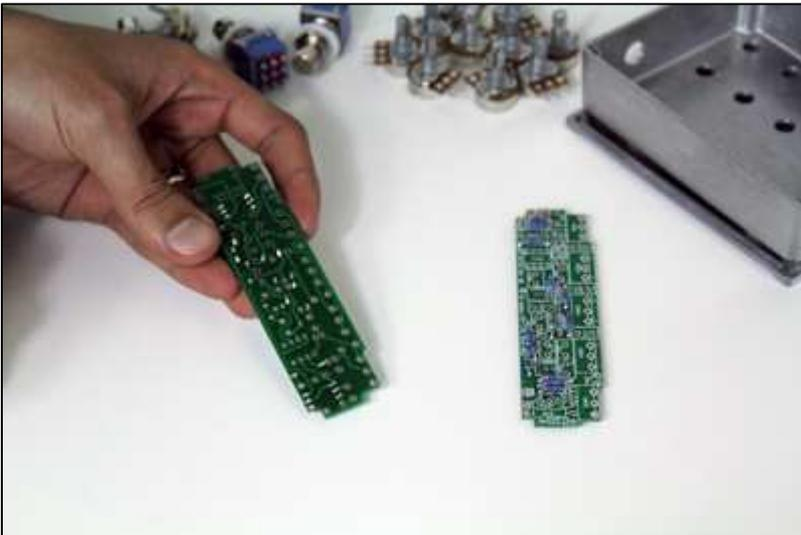
(4) Once all component legs are trimmed, inspect each joint to ensure its quality. Re-flow the solder of any suspect joints and double-check the value of components and position if you haven't already done so.
