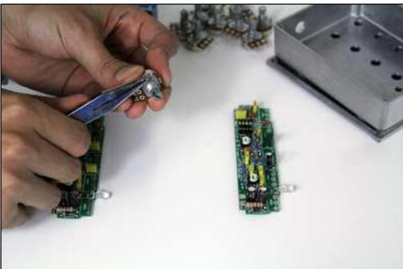
(14) Nearly there! Next to load are the potentiometers. Each pot has a small tab on the body (pictured). This will need to be snapped off with a set of needle-nose pliers or cutters. This will ensure the PCB will mount flush with the pedal case. All ten pots will need the tabs removed.
