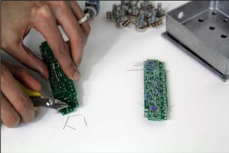
(3) Trim the component “legs” with a diagonal/side cutter. Try and cut as close to the board as possible without cutting off any of the solder joint.
