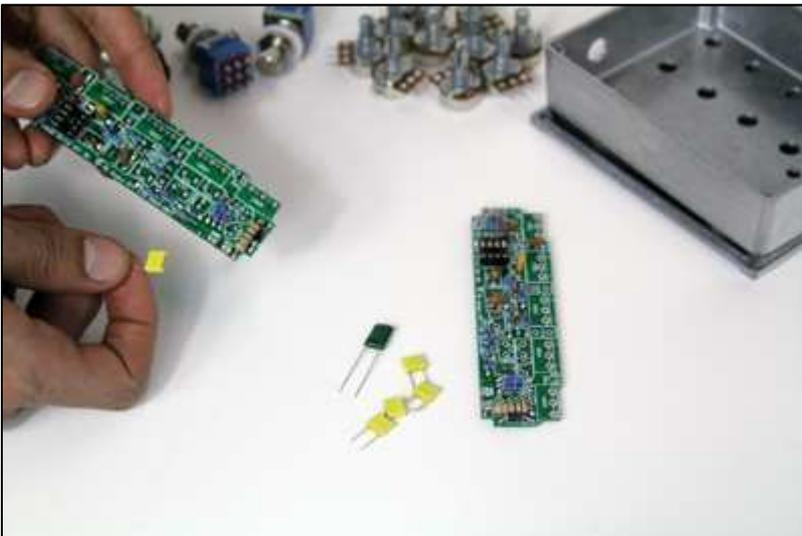
(10) The yellow and green film capacitors are next. These need to be sorted using their printed codes and are non-polarised. Place, solder, trim.
