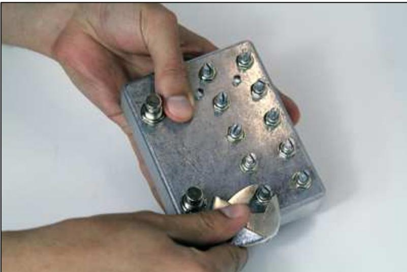
(22) Tighten the pots using the included nuts and washers, and ensure each pot is properly secured.
