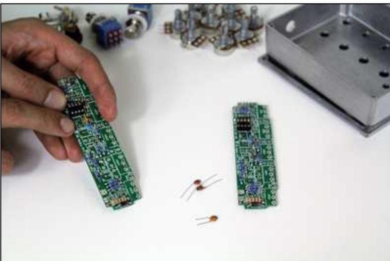
(8) Once all eight pins of the IC socket have been soldered, we will load in the ceramic capacitors. These will need to be sorted via their codes and placed in their positions. These are not polarised so they may be placed in either direction, regardless of the print on the circuit board.
