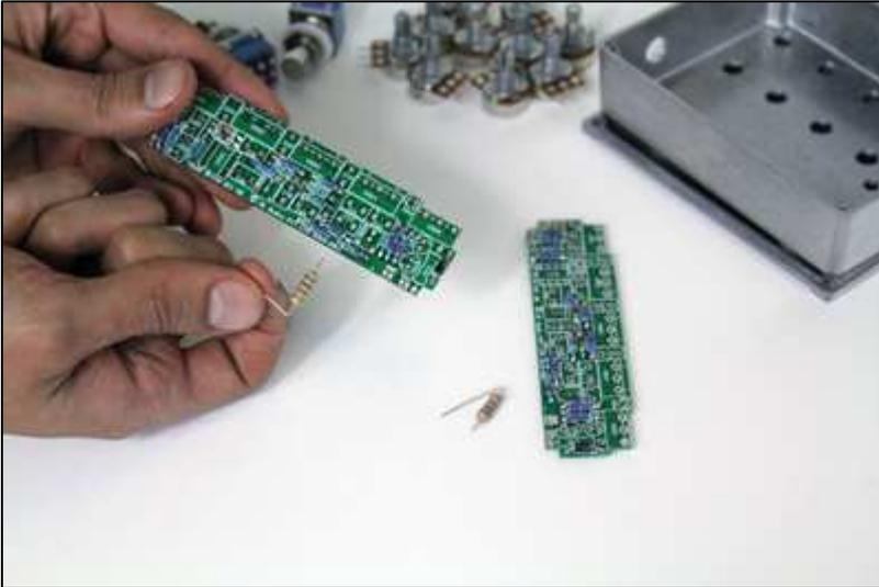
(6) Next to load is the large  $100\Omega$  1W, carbon film current limiting resistor.
