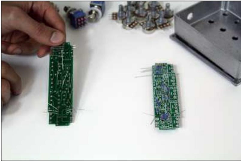
(1) Load in resistors first. Once you have determined each of their values via a multimeter or colour code and have clearly labelled them, begin loading as per designator for each PCB, A and B. You will need to straighten the legs of the resistor and re-bend to fit the PCB spacing length.
