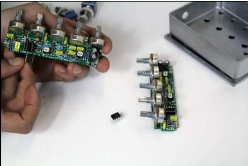
(16) Finally, we can load in the IC into its socket. Remember how the socket had a notch to denote its orientation? We want to load the IC in the same way, with the notch facing the same direction.
