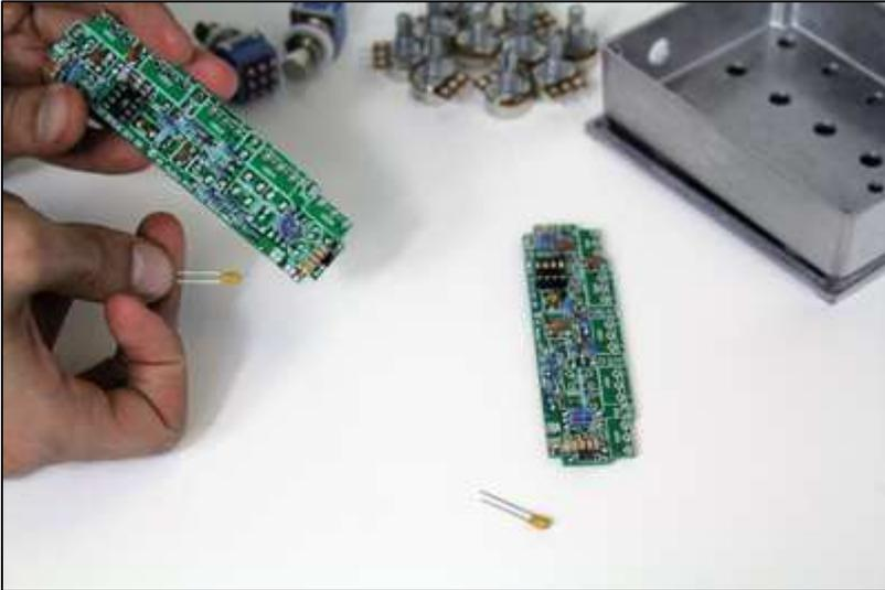
(9) Next up is the tantalum capacitor. This is polarised and the positive side is marked via two features; the side with the long leg is positive, and there is also a '+' marked on the cap itself. Place, solder and trim.
