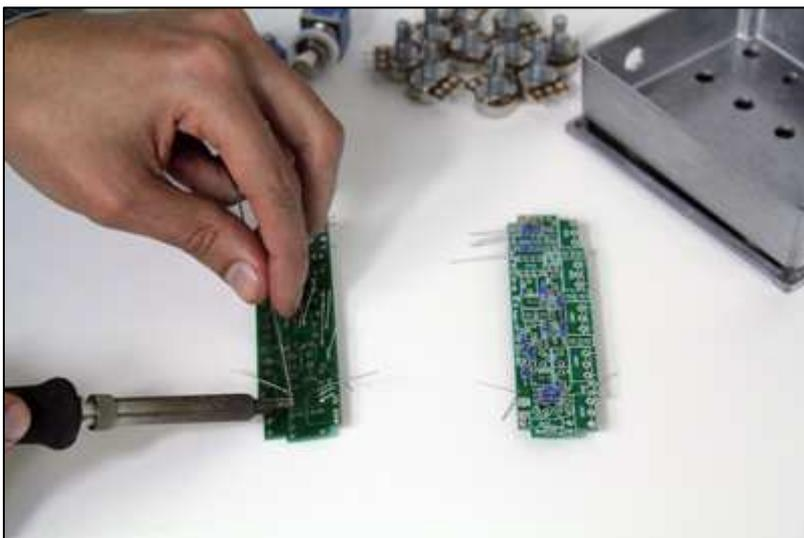
(2) Turn over and pay attention to each solder joint. The higher the quality of the iron, the better the solder will flow and form proper joints – that is it should be conical in shape, glossy and have no holes or cracks.
