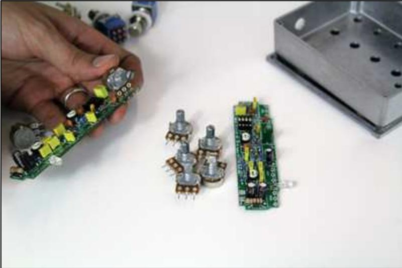
(15) Each pot is to be loaded facing away from the PCB as shown left. Load and solder in place but take care in not bending the pots back and forth whilst soldered.
